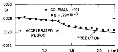
FIG. 6. Prediction of Stanton numbers in an accelerated fully rough boundary layer developing over uniform spheres roughness.
