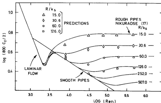
FIG. 1. Prediction of Nikuradse's [17] pipe skin friction coefficient data.
