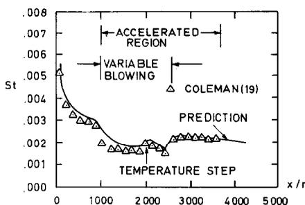
FIG. 7. Prediction of Stanton numbers in a fully rough boundary layer developing over uniform spheres roughness with acceleration, steps in blowing, variable blowing, and a wall temperature step.
