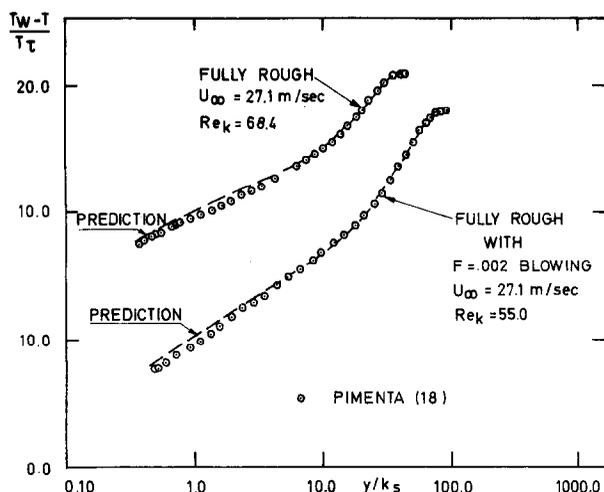
FIG. 5. Prediction of mean temperature profiles in boundary layers developing over uniform spheres roughness.
