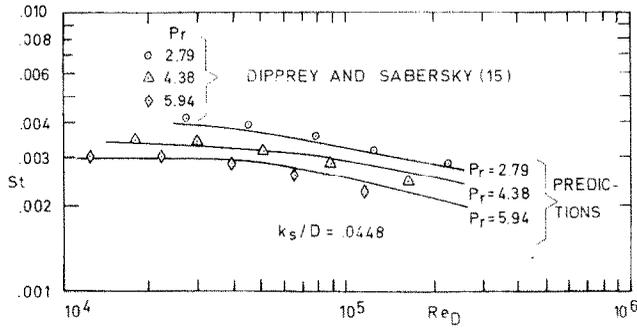
FIG. 2. Prediction of Dipprey and Sabersky's [15] pipe heat transfer data.
