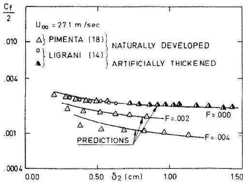
FIG. 3. Prediction of skin friction coefficients in boundary layers developing over uniform spheres roughness.
