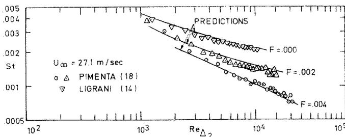
FIG. 4. Prediction of Stanton numbers in boundary layers developing over uniform spheres roughness.
